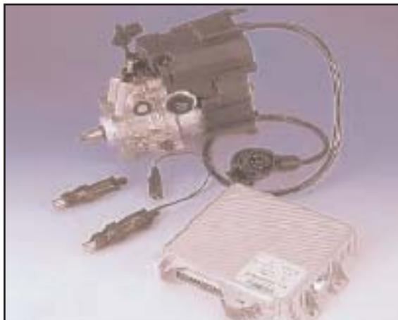
**Typical Applications** – The Delphi EPIC diesel fuel injection system is currently available for indirect injection engines where injection pressures are up to 350 bar, and direct injection engines where injection pressures of up to 950 bar are necessary.
